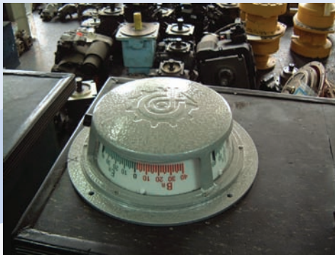
Rudder angle indicator for ceiling mounting, with light.
